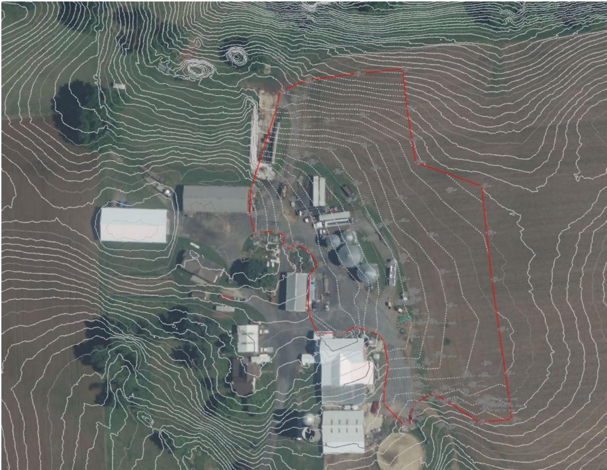
This shows the Surveyed Surface (Inside the red line) and the LiDAR Surface (Outside the red line) displayed together
