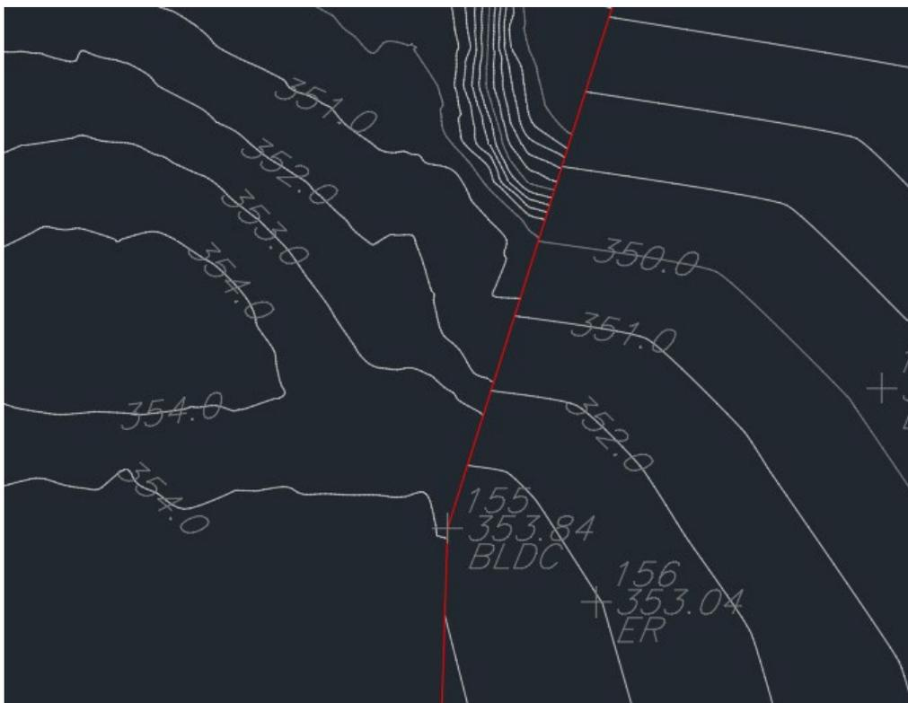
Now the LiDAR elevations match closer to the surveyed points elevations
