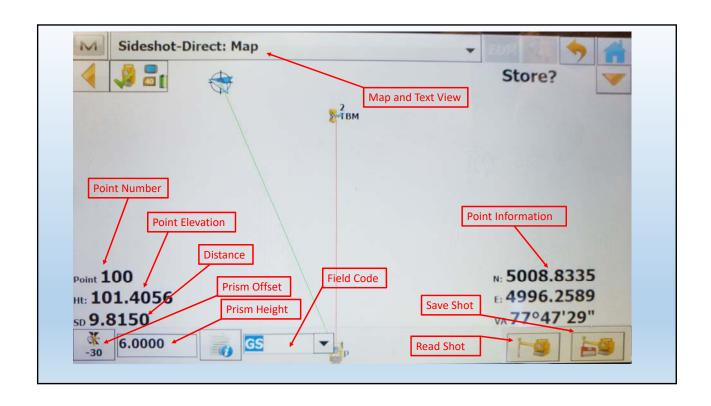
Adjusting the display on the TopCon FC-5000 Magnet Software V5.0 2018
